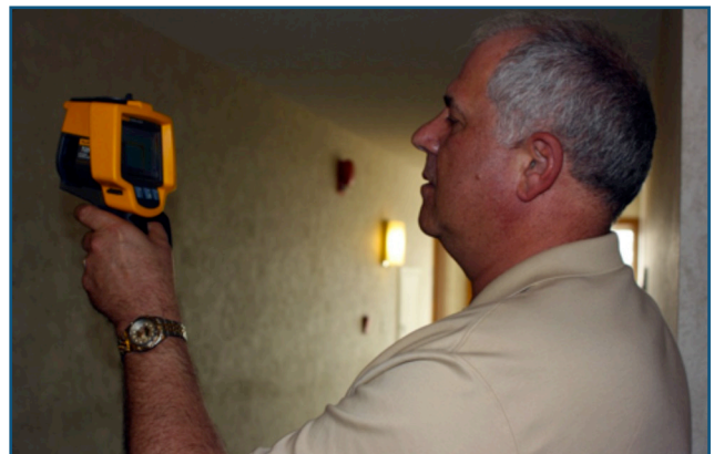
A pest management professional checks his infrared thermometer, used to check rooms for cold spots during heat treatments for bed bugs.
